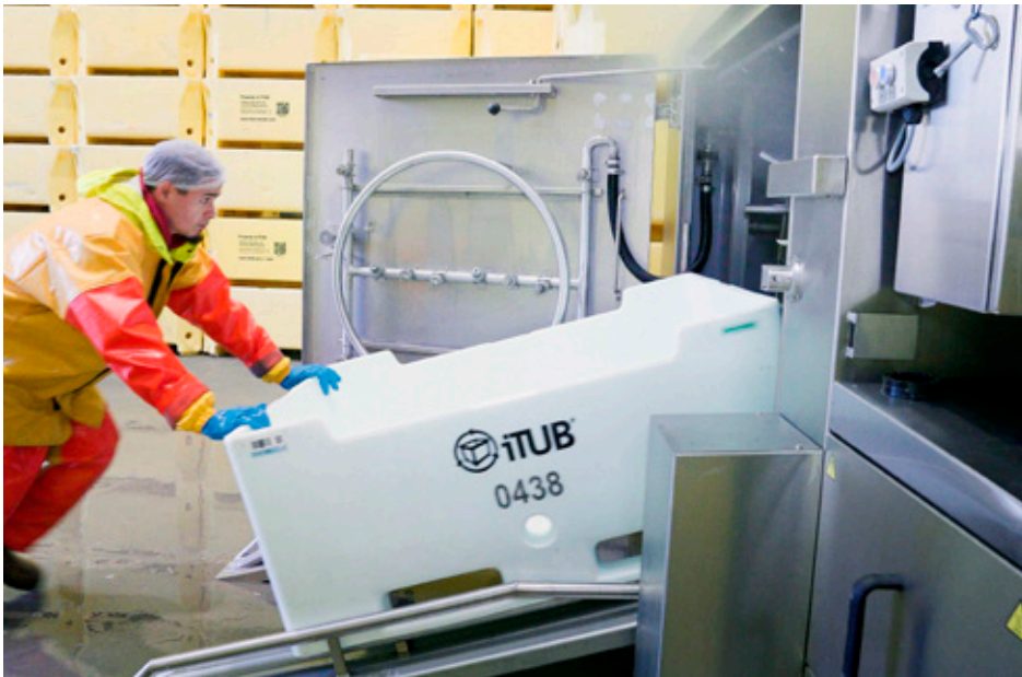
Once products reach their destination, tubs go to the nearest iTUB washing station to be cleaned and returned for the next shipment of farmed salmon.
